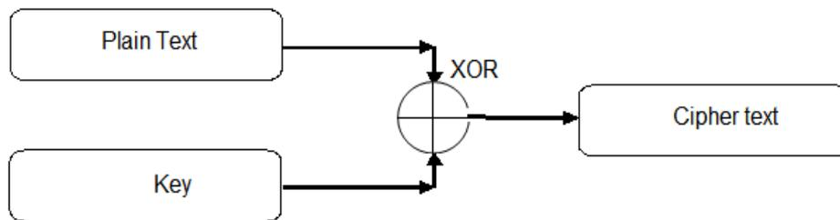
Figure 3: Block diagram of the. XOR encryption process
